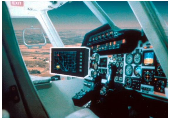
The GPS-enabled moving map display located in Mayo One's cockpit to show the helicopter's location on the displayed maps.
