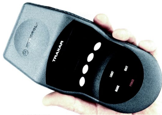
The Motorola Traxar handheld, six-channel GPS receiver distributed to law enforcement officers in initial work on the Mayo One helicopter project.
